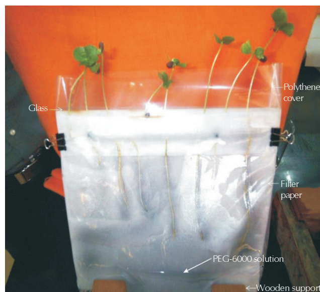
Figure 1: General view of the slanting glass plate technique experiment
